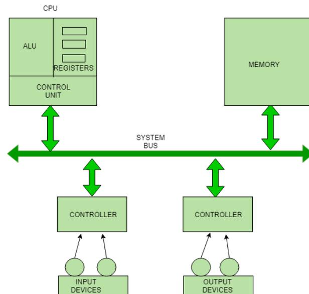
The address bus carries the address location of the data or instruction. The data bus carries data from one component to another and the control bus carries the control signals. The system bus is the common communication path that carries signals to/from CPU, main memory and input/output devices. The input/output devices communicate with the system bus through the controller circuit which helps in managing various input/output devices attached to the computer.
