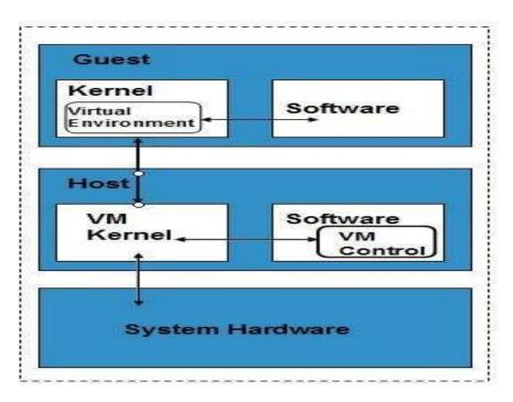
VMware vSphere is highly developed infrastructure that offers a management infrastructure framework for virtualization. It virtualizes the system, storage and networking hardware.
