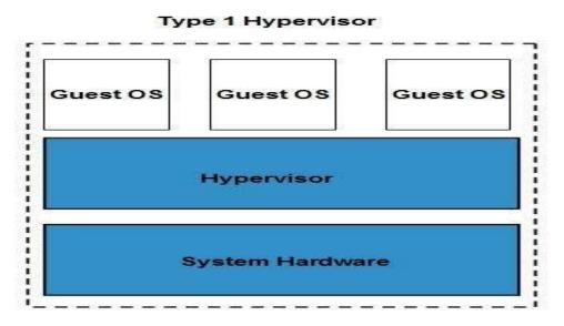
The **type1 hypervisor** does not have any host operating system because they are installed on a bare system.
